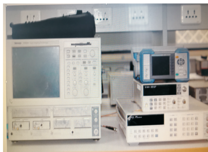
图 1 示波器校准仪检定装置组成 Fig. 1 Composition of calibration device for oscilloscope calibrator
